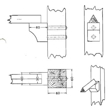
Supports for Pole Vault.—At competitions in Pole Vault, pegs shall be used for the support of the cross bar. The pegs shall be without notches or indentations of any kind, of uniform thickness throughout, and not more than 13 millimetres (½ inch) in diameter, and must not extend more than 75 millimetres (3 inches) from the uprights.
